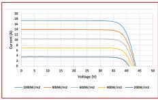
4) Average relative efficiency reduction of 5% at 200 W/m² according to EN 60904-1.
