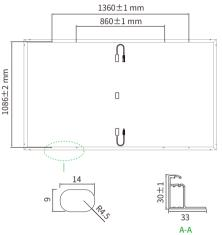
\*Note: For specific dimensions and tolerance ranges, please refer to the corresponding detailed module drawings.
